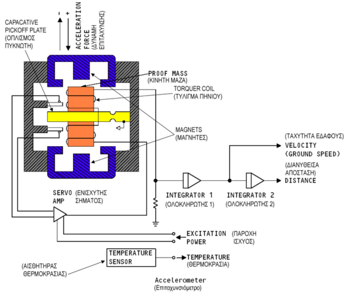
Typically, accelerometers use **linear sensors**: the output is (ultimately an electronic) signal proportional to the instantaneous acceleration.
