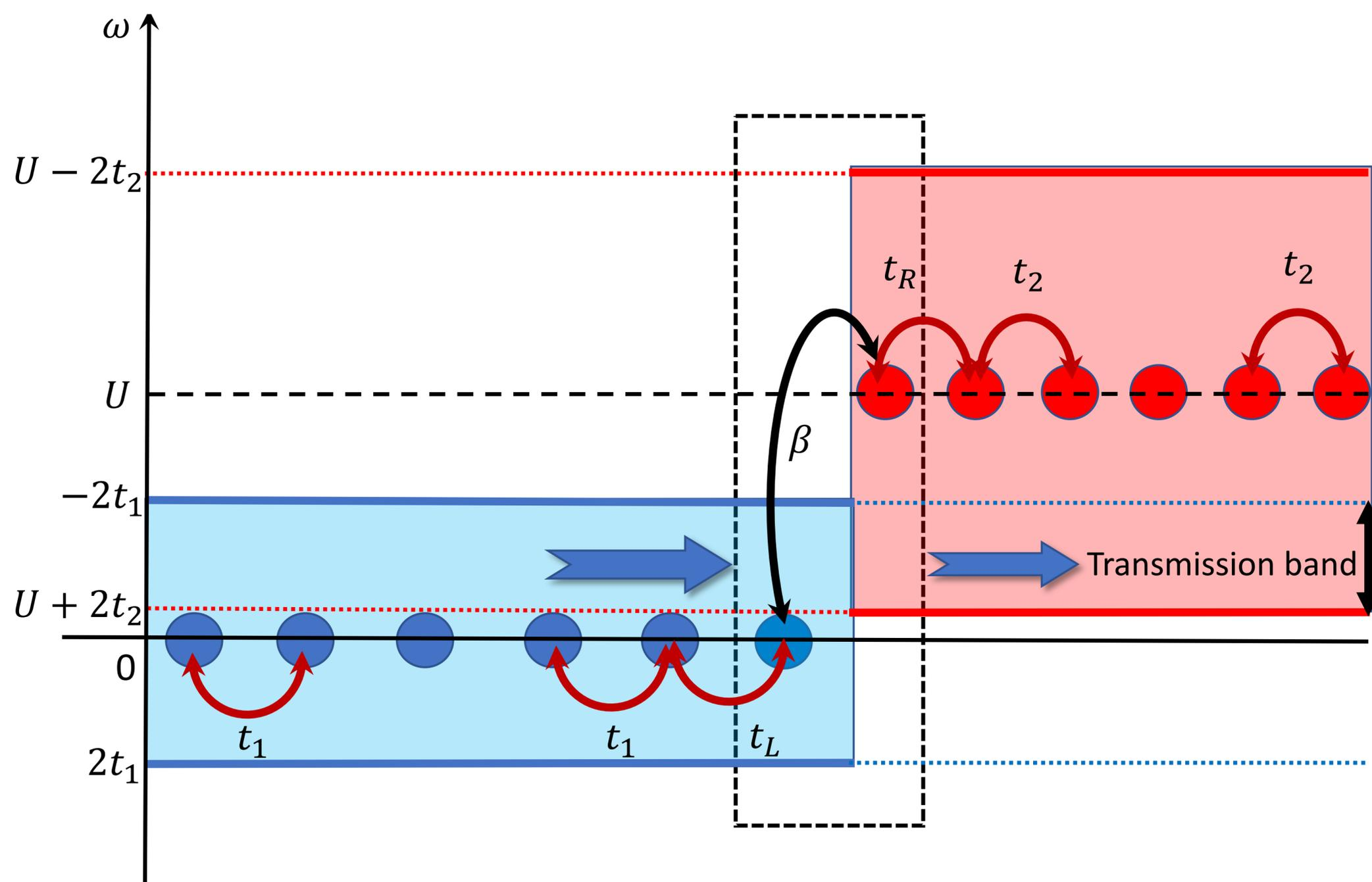
Figure S3: **Schematics of the CROW array interface.** Left/right CROW transmission lines are shown by blue/red resonators (see also Fig. 1D of the main text). The supported bands of the left/right transmission lines are shown by the blue/red region. The black vertical arrow indicates the region where the bands overlap forming a transmission band of the interface. The black dashed box indicates the system described by the Hamiltonian  $H_0$ .
